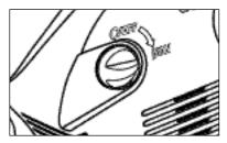
Step 6 Turn on the pressure washer (I). The motor starts only if the trigger of the gun is pulled and shuts off when the trigger is released.
